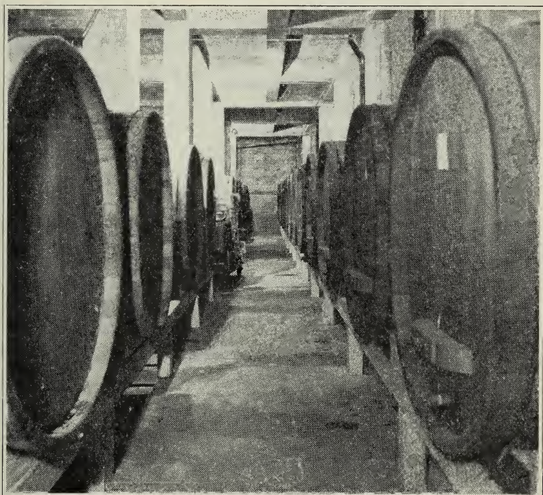
Fig. 14.—Storage tanks. Usually these are placed on end. Note the racking valve in the manhole. (Photograph by courtesy of the Wine Institute.)
